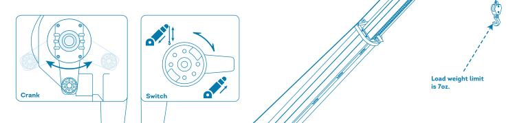
Turn support leg to lock and unlock in open and closed positions.
